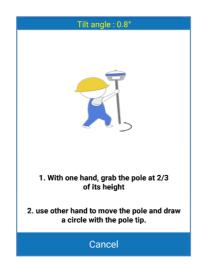
The second screen lets the sensor adjust the calibration parameters based on the local GNSS position and accuracy.
