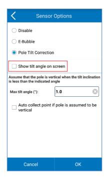
The user can also define the verticality tolerance of the instrument.
